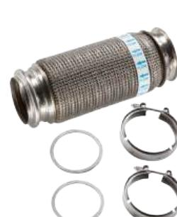
Manufactured with high temperature stainless steel 4 layer construction: liner, double layer corrugated material & a stainless steel mesh cover.
