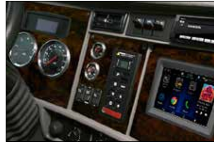
Easy-to-operate dash control panel for Eaton automated and Allison automatic transmissions.
