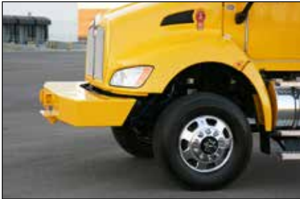
Factory installed front drive axles with capacities from 10,000 to 16,000 lbs. Non-driving front axles from 8,000 to 20,000 lbs.
