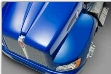
The four-piece hood and fenders are molded from SMC, a high-tech light weight composite material for added durability and reparability.
