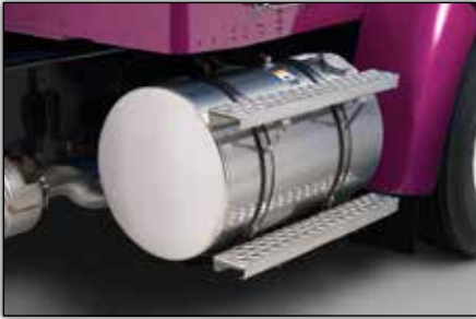
Kenworth-built polished aluminum fuel tanks in multiple diameters and capacities to meet your needs. New options include end of frame between rails fuel tanks.
