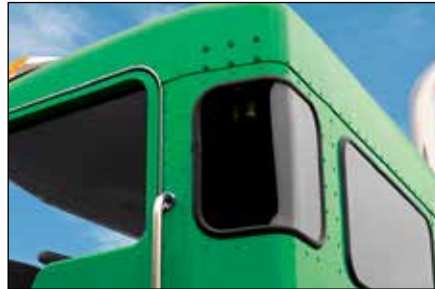
In addition to the standard peeper window in the passenger door, optional cab corner windows are available to help improve visibility in tight places.
